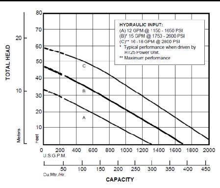
Curves are based on pumping water at 60°F. For performance curves other than shown above, consult factory.
