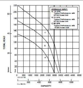
Curves are based on pumping water at 60°F. For performance curves other than shown above, consult factory.
