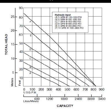
Curves are based on pumping water at 60°F. For performance curves other than shown above, consult factory.
