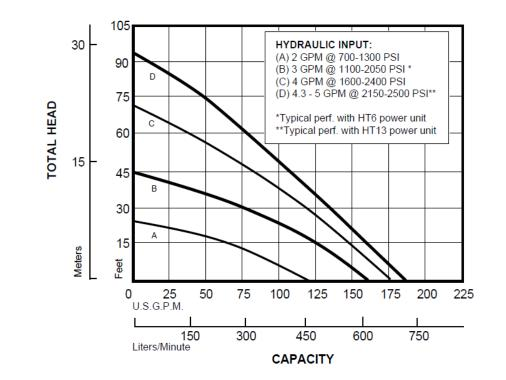
Curves are based on pumping water at 60°F. For performance curves other than shown above, consult factory.
